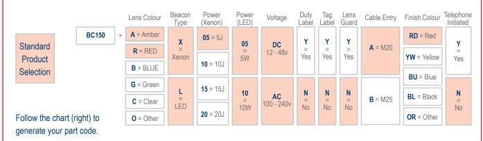
MODEL CONFIGURATOR (By using the table above, complete this box sequence to select your required beacon).
