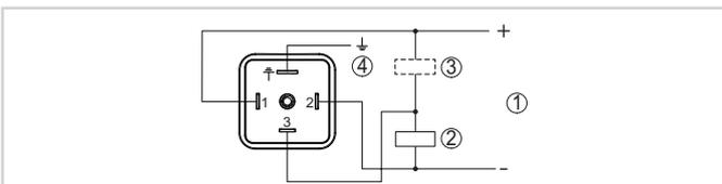
Wiring plan ISO 4400 plug - Transistor output, three-wire
