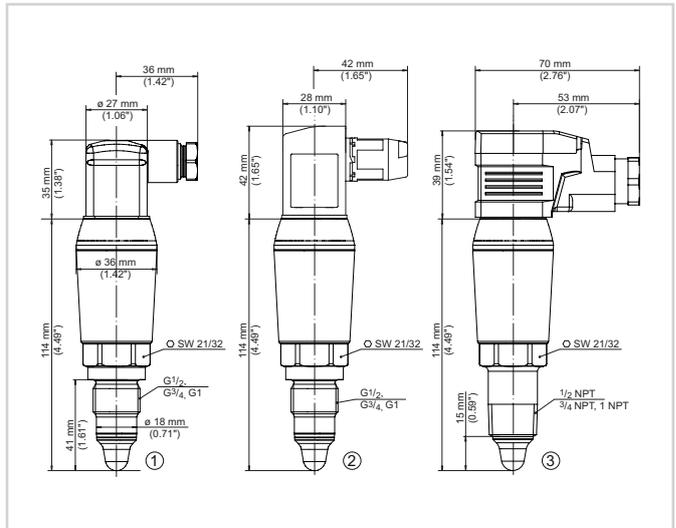
VEGAPOINT 31, standard version - thread with valve plugs acc. to ISO 4400
