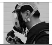
**13.**Connect the demand valve with the mask. Align the bayonet of the mask with the interface of the demand valve and press hard. The demand valve is securely connected with the mask when a "click" is heard.
