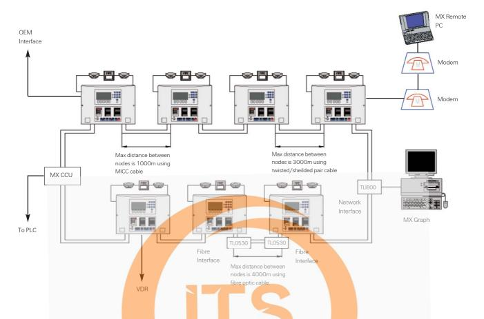
Up to 99 MX/T2000 sub-panels can be linked together providing unrivalled design flexibility (T2000 Only).
