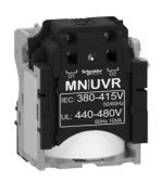
MN undervoltage release, ComPacT NSX, rated voltage 380/415 VAC 50/60 Hz, 440/480 VAC 60 Hz, screwless spring terminal connections
