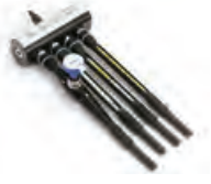
Adapter with Impactor connected in Dräger Aerotest Simultan
