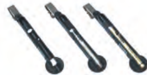
Dräger-Diffusion-Tubes with direct indication
