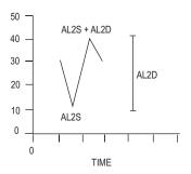
RL15 sets the relay on point, and RL15 - RL10 sets the relay off point. The relay's output functions in the direct acting mode, which means the relay activates with an increase in pressure. In the above graph, an instrument with a 50 psi range has the RL15 set at 40. The relay will turn on at 40 psi increase. The RL10 is set at 30. The relay will turn off at 10 psi decrease (40 - 30 = 10).
