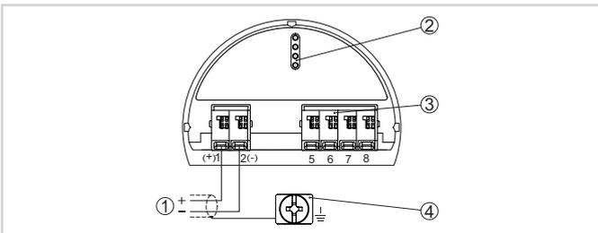
Secondary terminal connections (intrinsically safe devices)
