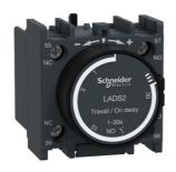
Time delay auxiliary contact block, TeSys D, 1NO + 1NC, on delay 1-30s, front, screw clamp terminals
