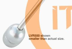
The LVR500 Series float level transmitter provides continuous level measurement up to 2 m (6.5') with a 4 to 20 mA signal output, and is factory configured to your selected dimension. This stainless steel liquid level sensor is well suited for high temperature or pressure tank level applications with relatively clean liquids such as water, diluted chemicals and light weight oils. Typical application examples include boilers and process vessels.
