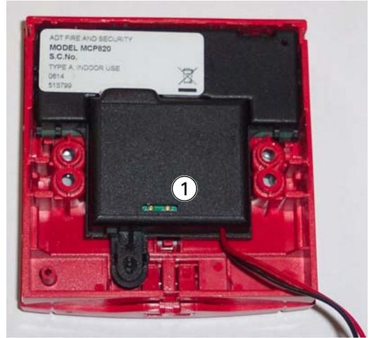
Fig. 3: CP820/CP820M - Address Programming Ports
