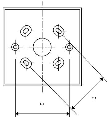
Fig. 2: CP820/CP820M Fixing Dimensions Surface Mounting
