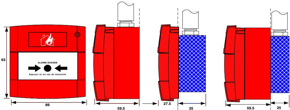
Fig. 4: CP820/CP820M - Overall and Fixing Dimensions
