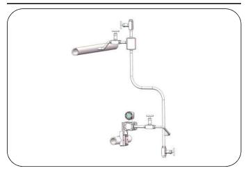
For high-temperature steam measuring, cooling water should be preinjected into the guided pipe, After the steam pipes are stable, slowly open the shut-off valve to start measuring.
