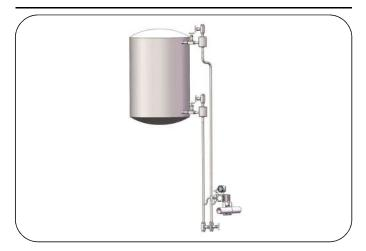
For sealed container level measurement, isolation tank and multiple shut-off valves should be used. Open the drain/vent valve periodically to clear the residual gas and liquid in the guiding pressure tube to ensure accuracy.
