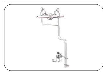
The pressure tube should be tilted up 45°, the installation location should be lower than the process pipeline. Isolation tank and multiple shut-off valves should be used. Cooling liquid should be pre-injected into the guiding pressure tube. The drain/vent valve should be opened periodically, clearing the residual gas and liquid in the guiding pressure tube to ensure accuracy.
