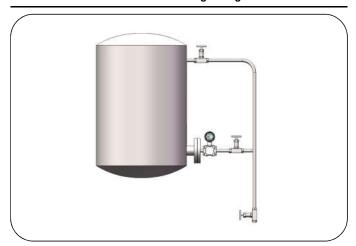
When single flange diaphragm system is used for sealed container level measurement, Isolation tank and multiple shut-off valves should be used, open the drain/vent valve periodically, clear the residual gas and liquid in the guiding pressure tube to ensure accuracy.
