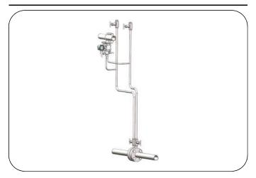
The pressure tube should be tilted up 45°, the installation location should be lower than the process pipeline. Isolation tank and multiple shut-off valves should be used. Open the drain/vent valve periodically to clear the residual gas and liquid in the guiding pressure tube to ensure accuracy.
