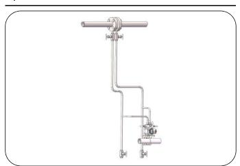
The pressure tube should be tilted down  $45^\circ$ , the installation location should be lower than the process pipeline. Isolation tank and multiple shut-off valves should be used. Open the drain/vent valve periodically to clear the residual gas and liquid in the guiding pressure tube to ensure accuracy.
