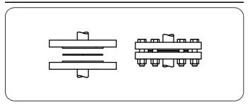
Choose gasket according to medium features and temperature range, pay attention to the bolt balance lock.
