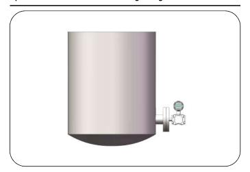
For open container level measurement, media compatibility should be considered, install on location where the liquid level and temperature changes stably to improve accuracy.
