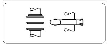
Choose gaskets which meet the health standards, to avoid excessive locking clamp and squeeze gasket and diaphragm and cause measuring error.
