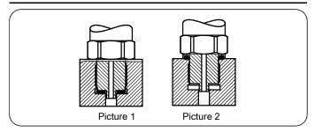
Picture 1: The length of pressure transmitter thread should be longer than the depth of the thread to ensure the seal of head face gasket is effective.
