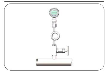
For high-temperature steam measuring, cooling water should be preinjected in the condenser filling the tube more than half way. After the steam pipes are stable, slowly open the shut-off valve to start measuring.
